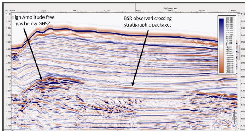
Figure 5: Pegasus Basin 2D far stack Line #06, location shown on basemap in Figure 3. Bottom simulating reflector clearly observed throughout this section as it cross cuts the stratigraphy.
