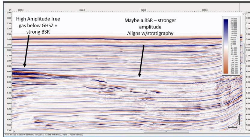
Figure 4: Pegasus Basin 2D far stack Line #19, zoomed into green box shown in Figure 3. Bottom simulating reflector is clear on the left of the seismic line where free gas is being trapped. A stronger amplitude is observed as compared to the full stack data in central region.
