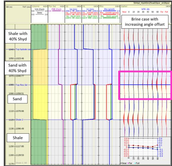
Figure 2: 4-layer rock model with amplitude vs. angle offset responses shown for a brine case. The amplitude response expected at the base of the GHSZ in a brine saturated reservoir sand is best observed at far angles.
