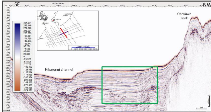
Figure 3: Pegasus Basin 2D full stack Line #19. Location map shows Line 19 location in red, and Line 06 location in purple. The green box highlights the region where the BSR at the base of the GHSZ is transparent.
