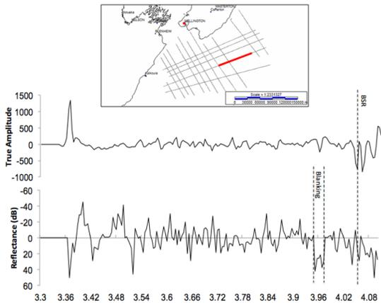
Figure 6: Initial calculated reflectance values in the region of the GHSZ for Pegasus Line #08 shown as the red line in map on top of figure. The BSR and interpreted amplitude blanking zone are identified with dashed lines.  $A_0$  was calculated at SP 3660, and  $A_i$  was calculated at SP 3172.
