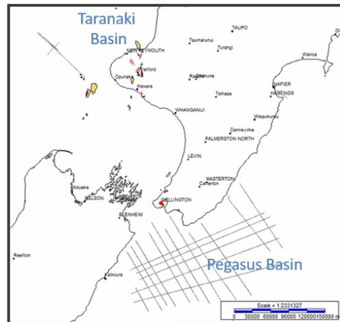
Figure 1: New Zealand study area, showing the location of 2D lines in the Pegasus Basin, as well as selected 2D lines in the Taranaki Basin. Producing petroleum fields in this region are also denoted by yellow and red polygons.
