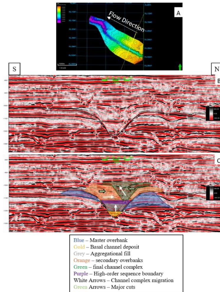
Figure 4: (A) Interpreted horizon picked for a master valley in the Pipeline-3D dataset. Paleo-flow direction is from the southeast to the northwest. (B) Arbitrary line seismic section displaying the interpreted channel complex. The location is shown in (A) by the yellow line. (C) Displays the interpretation of the channel complex along with the identification of architectural elements
