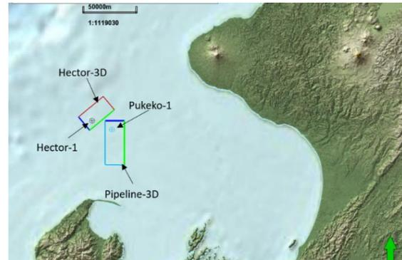
Figure 1: Map view of the study area. The seismic volumes are outlined along with the locations of the Hector-1 and Pukeko-1 wells.
